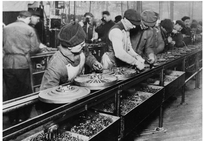
Fig.1: Workers on a T-model moving assembly line with magnetos and flywheels in 1913. Reproduced from Wikicommons [5].
